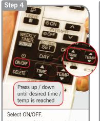
Make sure ON is selected and adjust the time and temperature by pressing the TIME and TEMP buttons.
