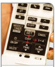
The buttons on the remote controller are set out in the order of how you set the timer. The clock on the remote must be set to the correct time.
